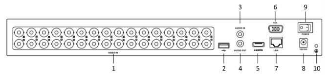
**NOTE** The rear panel of DVR-224Q-K2 provides 24 video input interfaces.
